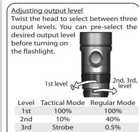
To switch between tactical and regular mode, turn on the flashlight at 1st level, dial to 2nd level and then back to 1st level for ten times within five seconds.
